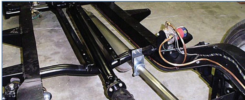
A typical, tough brake line routing path to which copper nickel provides an easier replacement solution.
